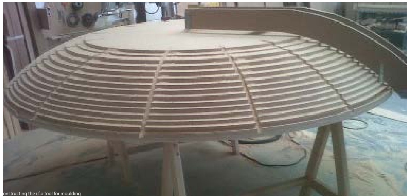
Constructing the i.f.o tool for moulding
